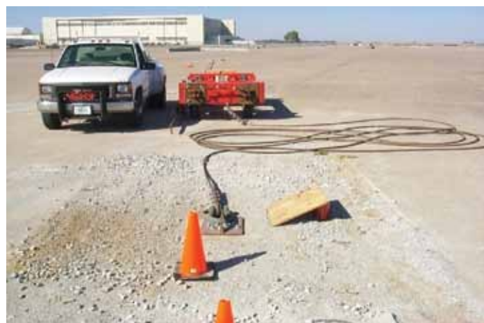
Cable Anchor Bogie Test Set-up
