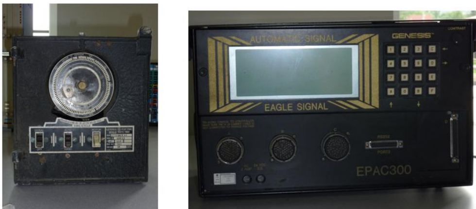
Figure 2. A 1940's vintage controller is on the left and on the right is a more modern controller.
